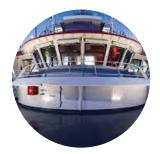
**Superstructure:** The non-sacrificial barrier created by Coval Marine blocks moisture, air, and chlorides to effectively prevent topside degradation due to salt-spray, galvanic corrosion, cathodic disbondment, and UV oxidation.
