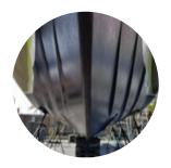
**Hulls:** Coval Marine's thin, hard, smooth surface reduces drag and help improve fuel efficiency without adding significant weight or displacement to the vessel; while acting as an antifouling, anticorrosion, antioxidation coating as well.
